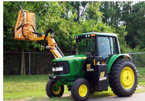
A-boom tracker used for trimming brush over guardrail and along side of the road with a 17 feet reach.
